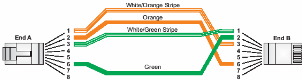
Figure B-3. Crossover Wiring
