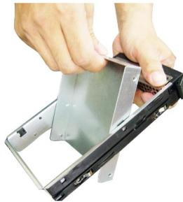
4. At the sides of the HDD are four screw holes, two on each side. Users will find on the HDD rack four identical screw holes as on the HDD. Place the HDD into the rack and align the screw holes on the HDD with the ones on the rack. Secure the HDD with four screws supplied by the HDD vendor.
