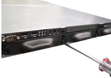
2. As the system mainboard supports two Serial ATA HDDs, only the HDD trays on the right & left sides can be used.
