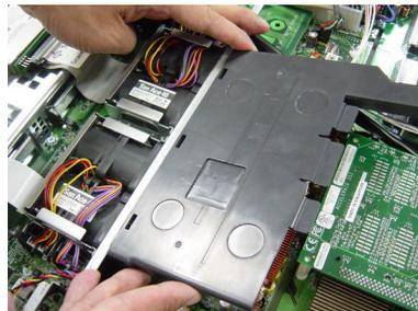
*Note: To ensure proper cooling, make sure the heatsinks & the fan duct are properly installed.*
