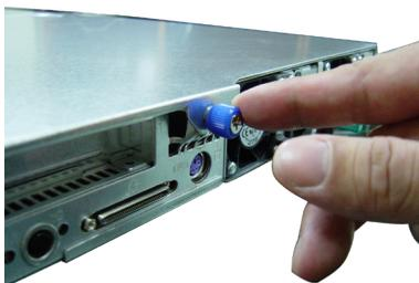
2. Press the release buttons and slide the rear chassis cover backwards to remove it from the chassis.
