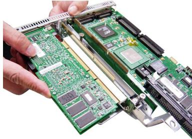
5. Place the riser card bracket on top of the PCI slots on the motherboard. Align the riser card golden fingers with the PCI slots. Then aim the front end of the riser card bracket at the standoff guide and align the rear part of the bracket with the U-shaped cuts on the chassis.
