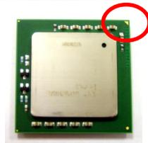
4. Place the CPU on top of the socket. Make sure to align the gold arrow on the CPU with the arrow key on the socket. Then push the lever down to secure the CPU in place.
