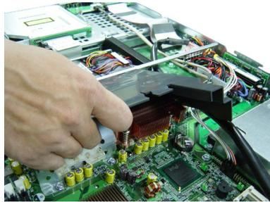
2. Locate the first CPU socket and raise the lever up to its full extent.
