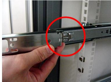
2. At the other end of the cable arm are two holes. Align the holes of the cable arm with the tabs on the rack rail (as indicated by circles and arrows).
