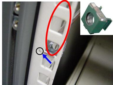
2. Align the rack rail with the rack and screw the rail to the rack by securing one screw to the bottom screw holder.
