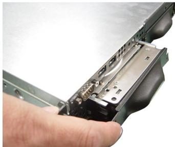
6. Screw the HDD set securely back to the system.
