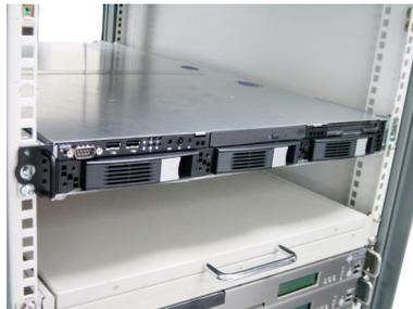
3. Screw the system firmly to the rack.
