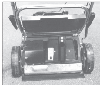
Figure 1 - Installing the Mulch Plug - 35m, 75m
