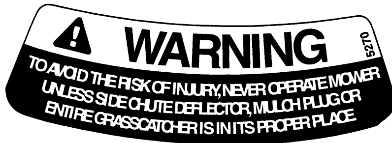
Figure 1 Safety Labels Found On Lawn Mower
