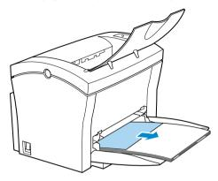
2 After removing a misfed page, be sure to open the top cover then close it again to reset the printer.
