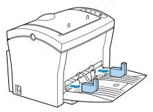
**5** Squeeze the right paper size guide and open the paper size guides. Pull out the plastic-lead strip from the paper feed inlet.
