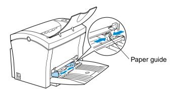
2 Place a stack of paper in the center of **Tray1**. Squeeze the right paper guide and adjust the paper guides so that both the left and the right sides of the paper stack are secure.
