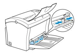
4 Place a stack of paper in the center of **Tray1**. Squeeze the right paper guide and adjust the paper guides so that both the left and right sides of the paper stack are secure.
