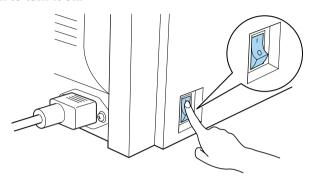
Turning on the printer causes all the indicators on the control panel to light, which indicates that the printer is warming up. In about 23 seconds or less, only the **Ready** indicator remains lit, indicating that the printer is ready to print.
