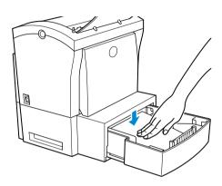
2 Remove the stack of paper from the tray and pull the misfed paper straight out of the printer.
