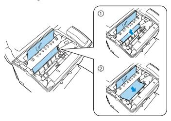
5 Reinstall the **drum cartridge** and **toner cartridge**. See "To Replace the Drum Cartridge" on page 6-7 and "To Replace the Toner Cartridge" on page 6-1 for details.
