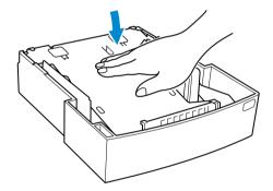
4 Place a stack of up to 500 sheets of paper into **Tray2** so that the side that was facing up when the paper was unwrapped is still facing up.
