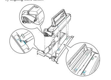
The cartridge will click into place when it is completely installed.
