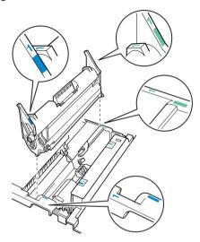
• Make sure the **drum cartridge** is inserted inside the printer as far as it will go.
