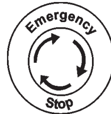
Figure 58. Emergency Stop Button
