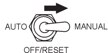
Figure 42. MPEC Control Switch (Manual Position)
