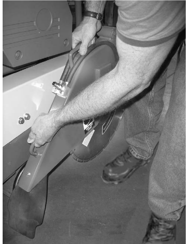
Figure 15. Removing The Blade Guard
