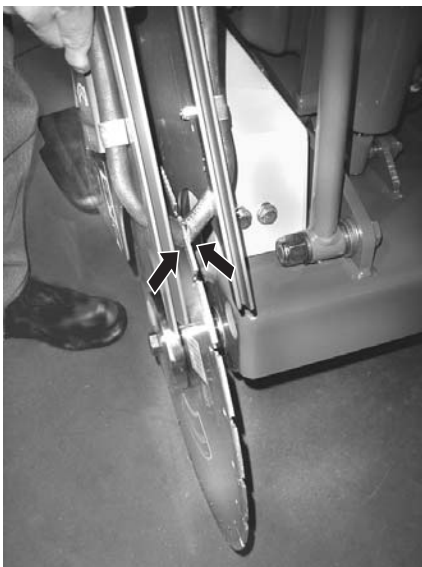
Figure 17. Water Hose Detail
