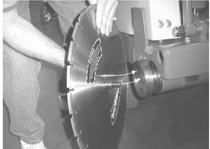
Figure 10. Aligning Flange Pin Through Blade
