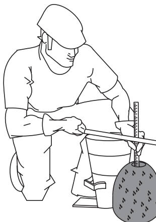
Figure 60-F. Slump Test (Measurement)
