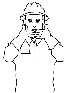
ALL DONE CLEAN-UP
