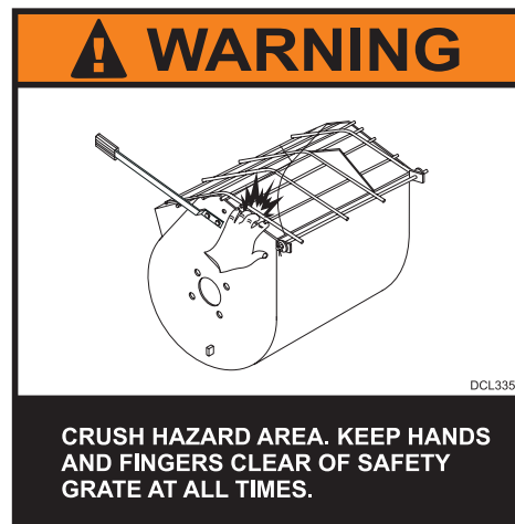
Figure 37. Safety Grate (Crush Hazard)
