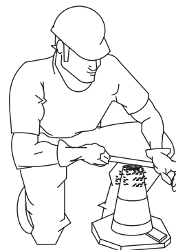
Figure 41-D. Slump Test (Removing Excess Concrete)
