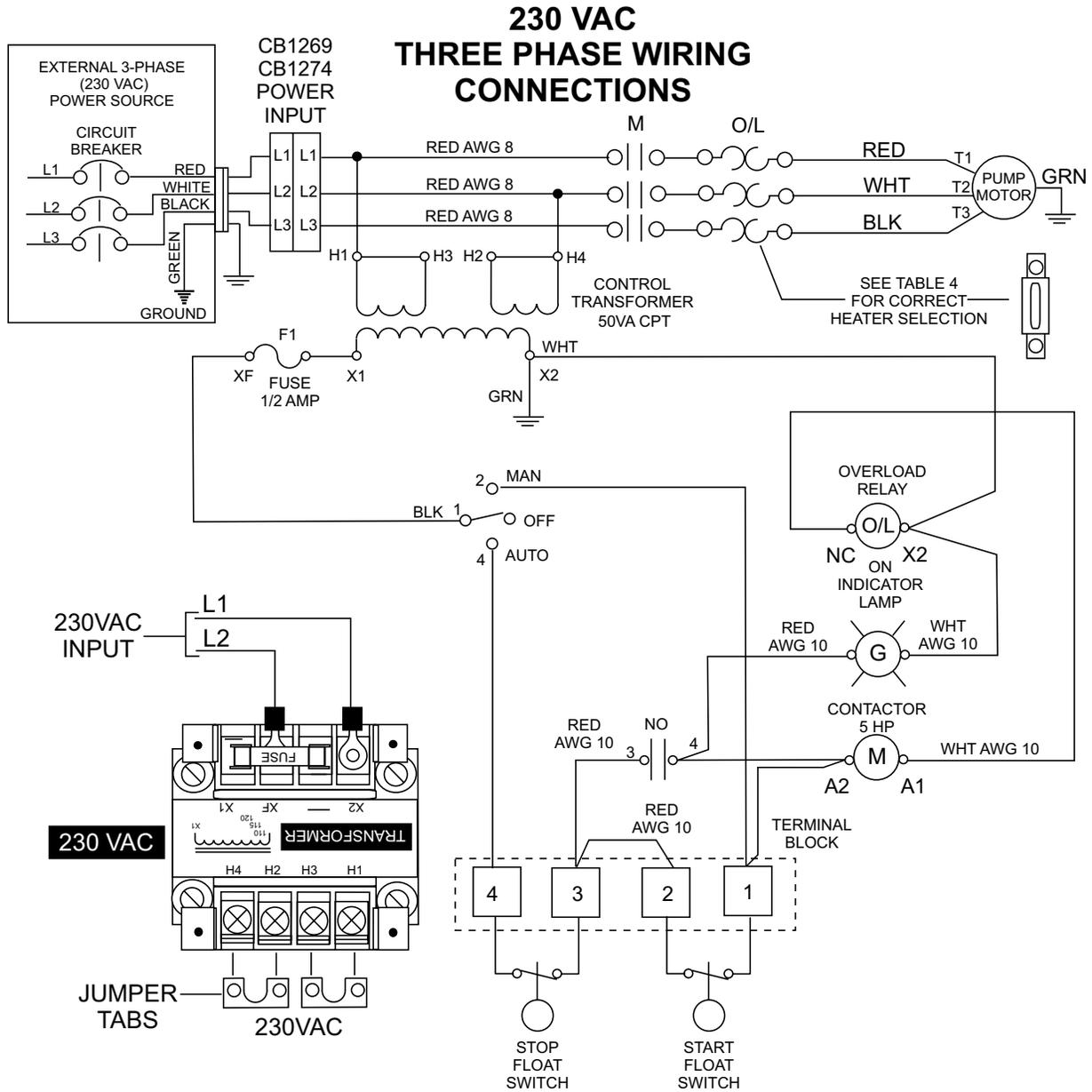
Figure 20. CB1269/CB1274 Control Box Wiring Diagram
