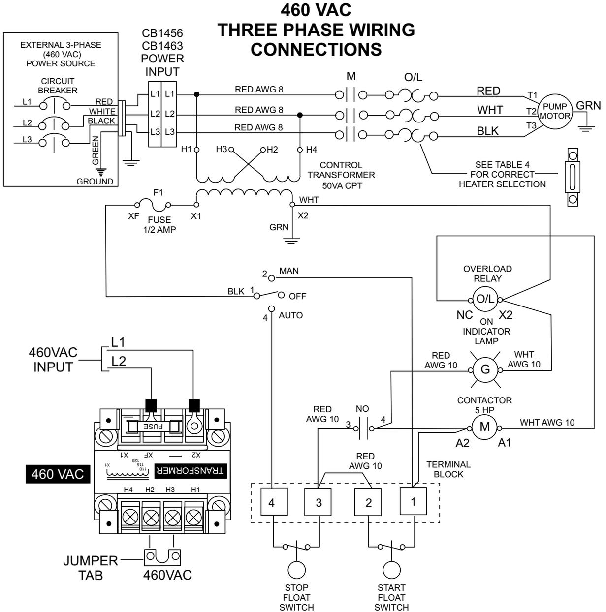
Figure 21. CB1456/CB1463 Control Box Wiring Diagram
