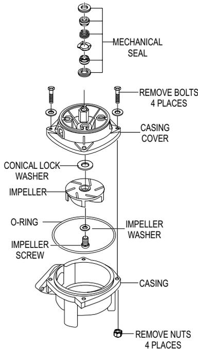
**Figure 20. Mechanical Seal Impeller Removal (PX400)**
