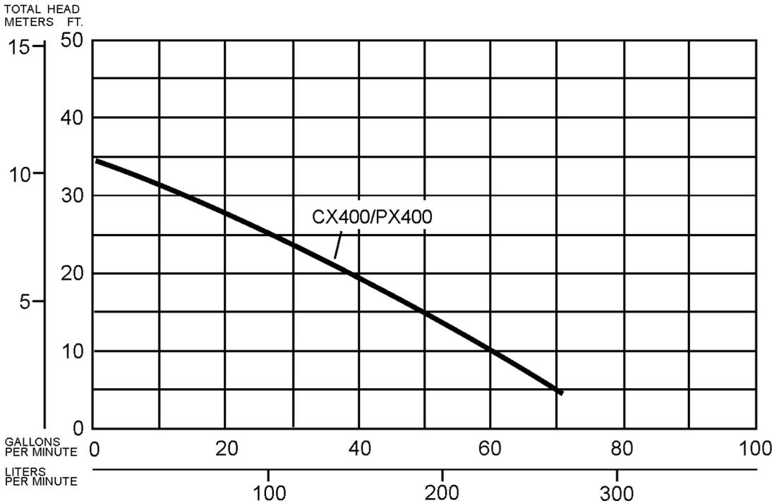
Figure 2. Pump Performance Curve
