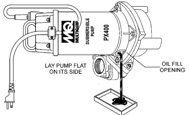
DISCOLORATION OF OIL (MILKY) INDICATES A WORN OR DEFECTIVE MECHANICAL SEAL. REPLACE MECHANICAL SEAL.
