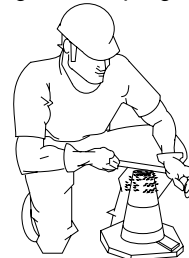
Figure Q. Slump Test (Removing Excess Concrete)
