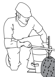
Figure S. Slump Test (Measurement)
