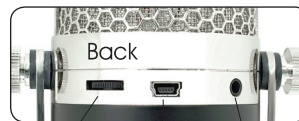
Analog gain controls USB Input Stereo headphone jack with high quality headphone amplifier
