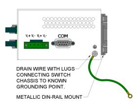
If the use of shielded cables is required, it is generally recommended to only connect the shield at one end to prevent ground loops and interfere with low level signals (i.e. thermocouples, RTD, etc.). Cat5e cables manufactured to EIA-568A or 568B specifications are required for use with N-Tron Switches.
