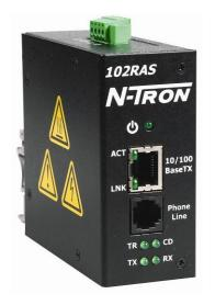
The N-TRON 102RAS provides connectivity to an industrial LAN for telecommuters or mobile users, or to remotely installed equipment, via an integrated V.92/56K modem. The small size of the 102RAS makes it ideal for placing alongside other industrial equipment to be accessed remotely.
