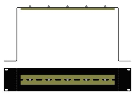
Most N-Tron<sup>™</sup> products are designed to be mounted on industry standard 35mm DIN rail. However, DIN rail mounting may not be suitable for all applications. Our Universal Rack Mount Kit (P/N: URMK) may be used to mount the 102RAS to standard 19" racks as an option.
