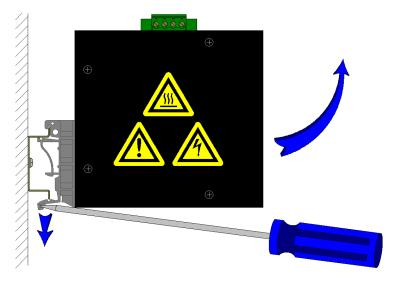
To mount the unit to the 35mm DIN rail, place top edge of the brackets on the back of the unit against the DIN rail at a  $45^{\circ}$  upward angle. Lower the bottom of the unit until it snaps into place on each bracket.
