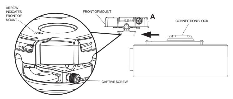
**IMPORTANT**: For security installations, insert one #10-32 x 1/4" socket pin screw (**D**) through projector mount assembly (**A**) and into connection block as shown in detail 1. Tighten screw using 4mm security allen wrench (**B**).
