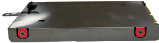
Fig. 4 Unscrewing the hard disk drive shield screws
