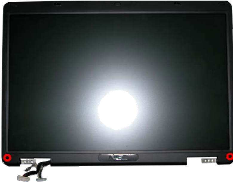
Fig. 25 Screws on the LCD Module
