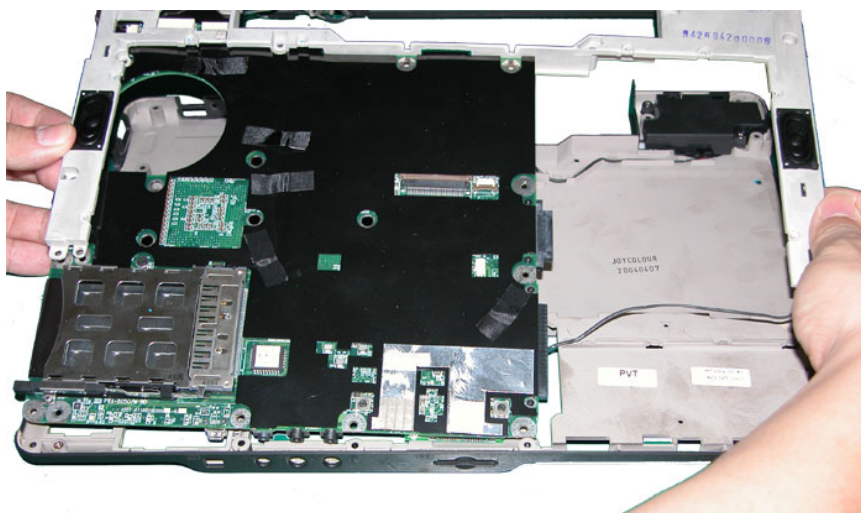
Fig. 32 Lifting up Main board
