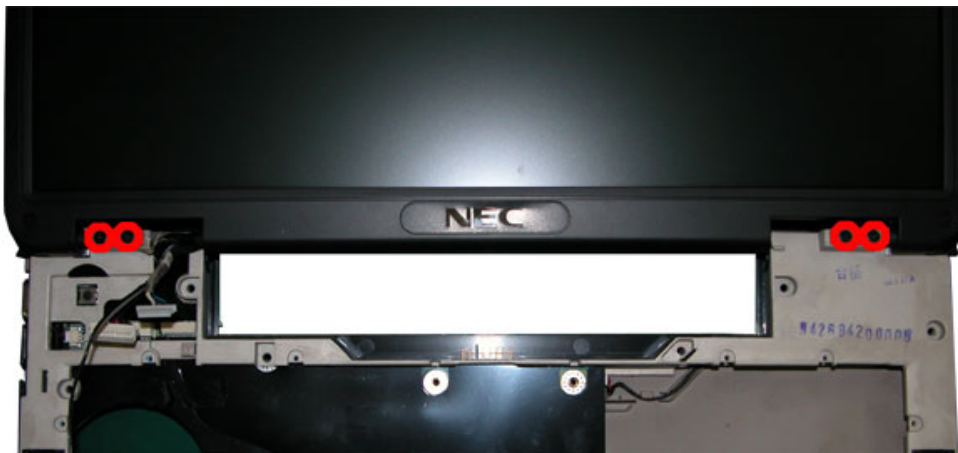
Fig. 24 Releasing the LCD Hinges
