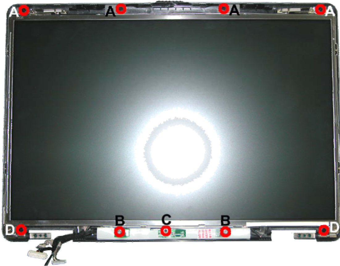
Fig. 27 Removing the LCD panel screws
