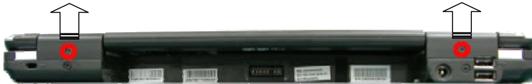
Fig. 21 Releasing LCD hinge cover
