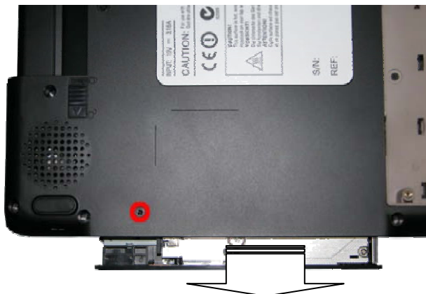
Fig. 6 Removing the optical drive
