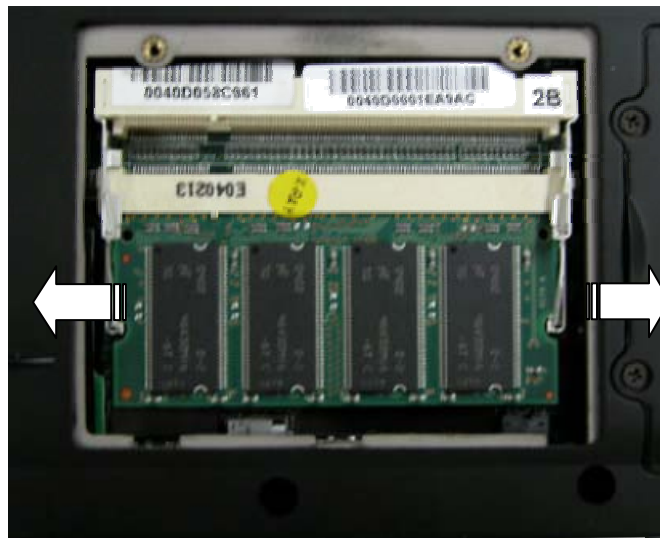
Fig. 8 Removing the memory module
