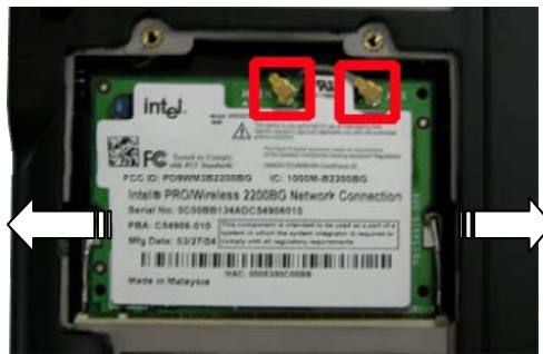
Fig. 10 Removing the WLAN module
