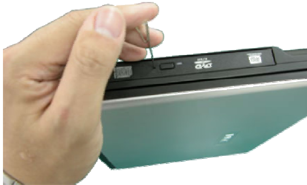
Fig. 5 Ejecting ODD tray
