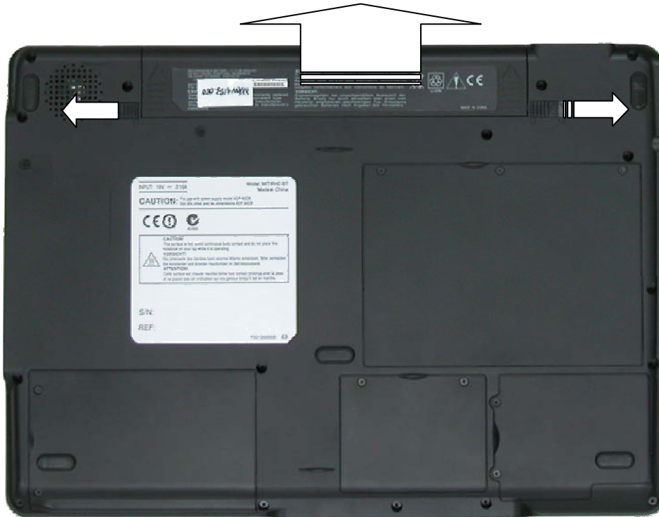
Fig. 1 Removing the battery
