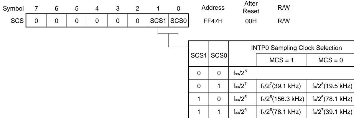
Figure 21-7. Sampling Clock Select Register Format
