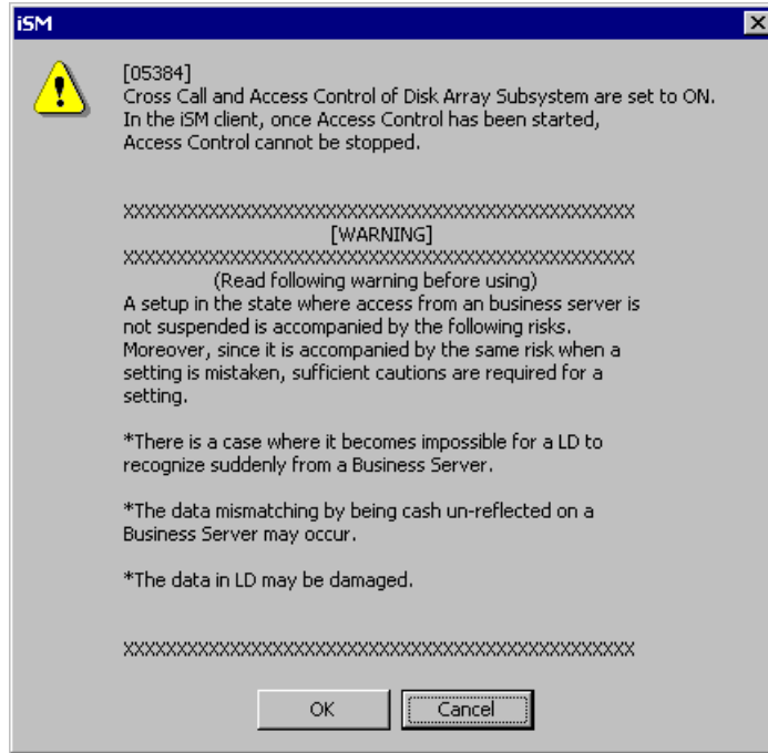
Figure 10-24 Start Access Control
