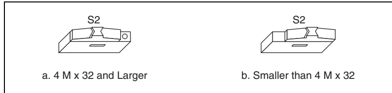
Figure 4-6. SIMM Size Configuration
