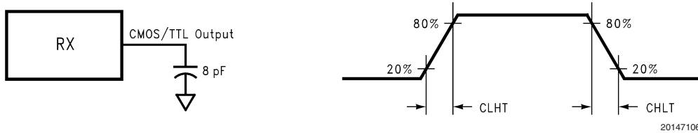
FIGURE 5. LVC MOS/LVTTL Output Load and Transition Times
