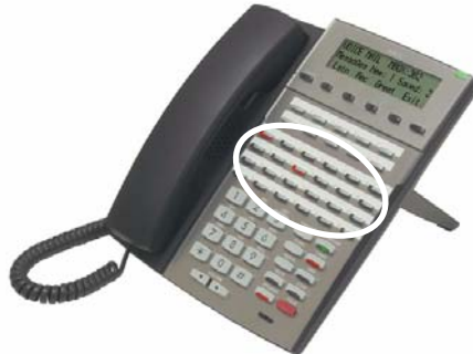
The 34-Button Display Telephone features 24 Feature Keys.
