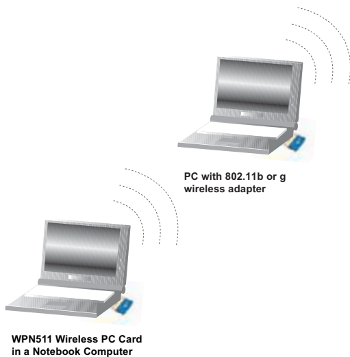
Figure 4-3: NETGEAR WPN511 Wireless PC Card in Peer-to-Peer Mode
