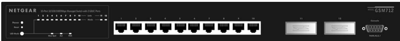
Figure 2-1. Front Panel of the GSM712 Managed Gigabit Switch
