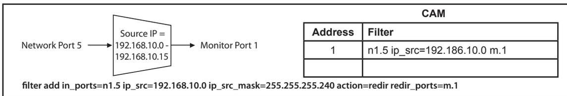
Figure 34: A simple IP address filter, shown with CAM
