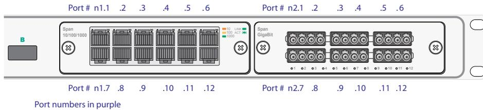
Figure 18: Port numbering for Span DNM models
