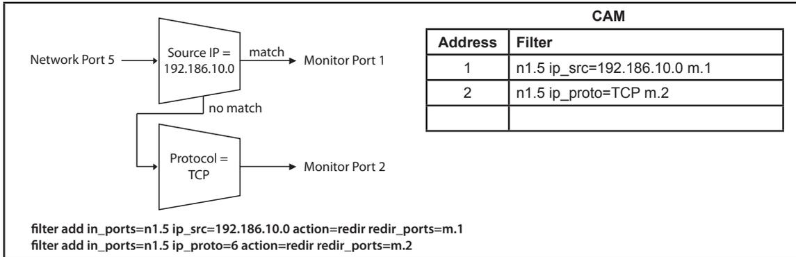
Figure 36: Correct flow diagram for two interacting filters
