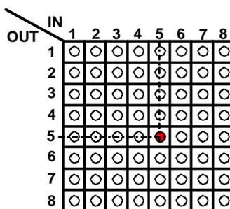
Figure 5- LED Matrix showing input 5 connected to output 5
