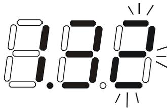
With the desired port number selected, point the IRT at the switch/receiver and press the "IN" button to transmit the selection and make the change. The blinking number in the LCD will stop blinking. The LED at the receiver will go OFF.
