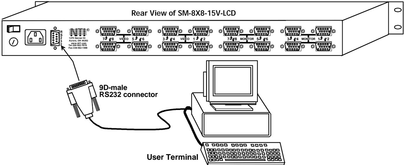
Figure 3- Connect user terminal for RS232 control
