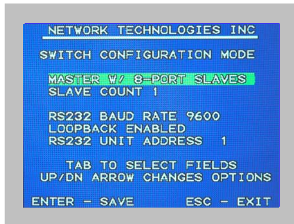
Figure 20- Switch configured as a master with one slave attached
