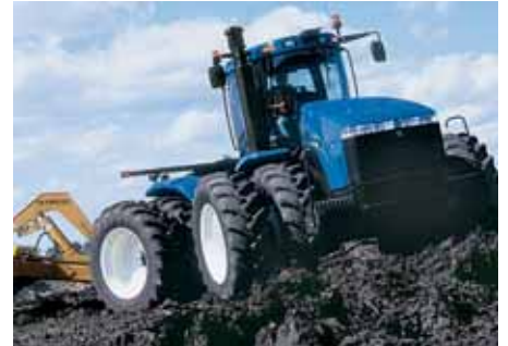
T9000 engines produce from 380 to 480 hp and also give you up to 40% torque rise and power growth of up to 54 hp. That's more than enough power and torque to pull the heaviest carry-all scraper.
