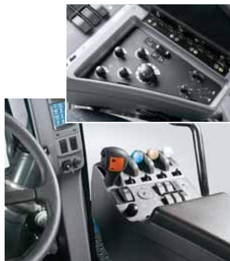
Right at hand . . . controls for AutoShift™ hydraulic remotes, flow and timer, diff lock, hitch, custom headland management, optional slip limit, throttle and gear selection are integrated into the armrest for ready, comfortable access.
