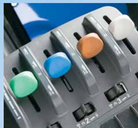
Hydraulic control levers and couplers are color-coded for ease of hook-up and to help track hydraulic operations.
