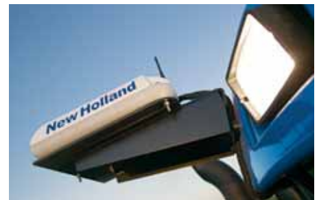
The New Holland 252 antenna receives the GPS signals to guide the vehicle. This antenna can easily be transferred from tractor to tractor or even to your combine.
