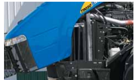
The cooling system provides the extra cooling capacity needed with higher-horsepower engines. The radiator is sized to the engine and can be accessed easily for cleaning.
