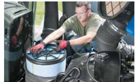
The large and extra-large frame tractors feature a new engine air intake system. The engine air filter has been relocated under the hood for a more efficient air flow and filter life.
