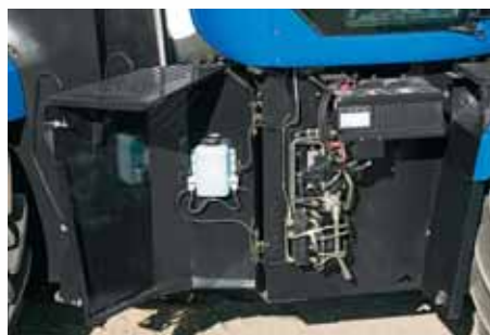
Reach batteries, washer fluid and axle lube filter through this handy right-hand service door. Steps on the door let you use a service-access window to reach the electrical components in the cab and easily route monitor cables.
