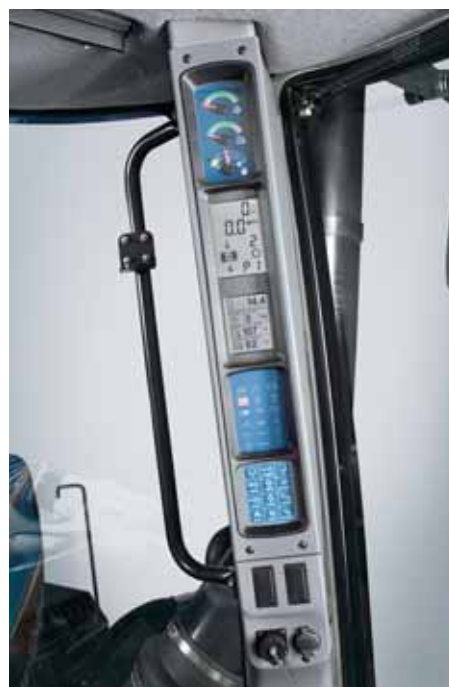
All the information you need on the go and at a glance — you can monitor everything from wheel slip and ground speed to fuel usage and hydraulic-flow readings with the optional performance instrumentation that's integrated into the cab post for easy viewing.
