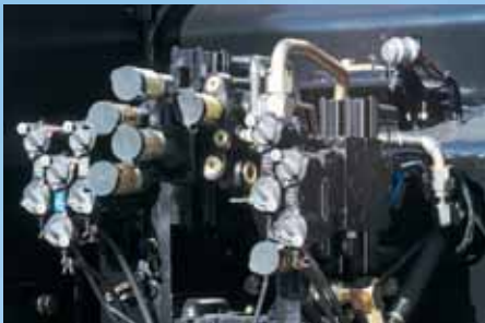
Up to 9 remote valves and MegaFlow™ can be built into any T9000 model. Seven remote valves and power beyond are pictured.
