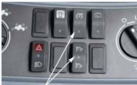
Use the constant speed switches to set the max RPMs and the speed adjustment switch or throttle to return engine speed to the desired level after making a turn.
