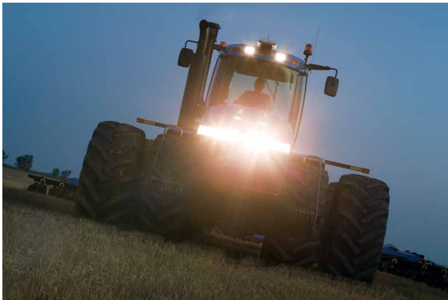
Halogen work lights, plus High-Intensity Discharge (HID) lamps, brighten the night. You can adjust eight of the work lights to focus more illumination on areas in front of, behind and to the side of the tractor.
