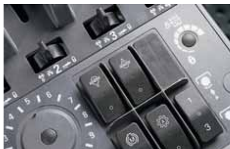
Differential locks have independent controls for front and rear axles.
