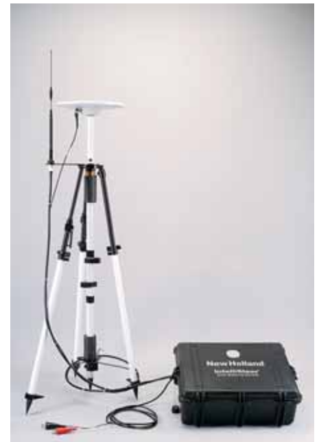
The RTK base station includes a GPS antenna, receiver and radio link to provide RTK correction signals to tractor-mounted auto-guidance systems and can be either portable or permanently mounted.
