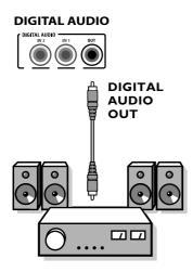
Connect a digital MultiChannel Surround receiver to the **DIGITAL AUDIO OUT** connector at the bottom of the TV.
