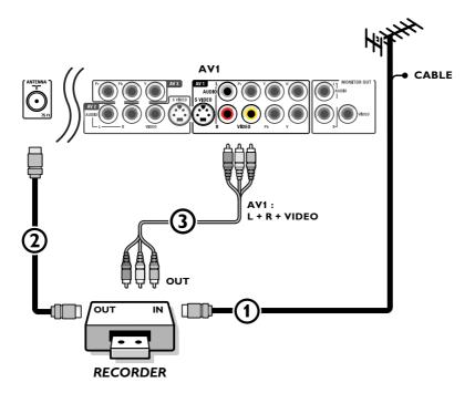
Note: Do not place your recorder too close to the screen as some recorders may be susceptible to signals from the display. Keep a minimum distance of 0.5 m from the screen.
