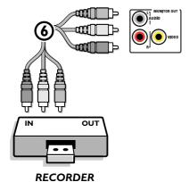
The **MONITOR OUT** connector can be used for a daisy chaining or to record programs from your TV **(()**. Only when a recorder is connected to **MONITOR OUT** it is possible to record an analog program from your TV. See Record with your recorder, p. 30.
