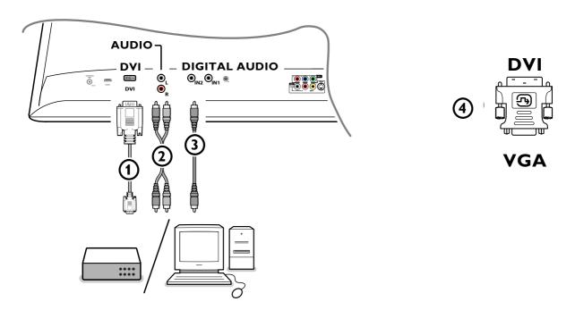
The **DVI** connector allows the following TV and monitor display modes, via the - key on the remote control, for High Definition (HD) and computer (PC) equipment:
