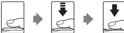
Press the shutter-release button halfway to set focus and exposure.
