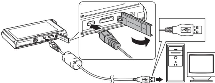
The camera is automatically turned on and the power-on lamp will light or blink. The camera monitor will remain off.
