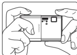
When taking pictures in portrait ("tall") orientation, turn the camera so that the built-in flash is above the lens.
