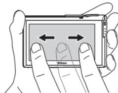
When the camera is in full-frame playback mode, drag two fingers across the touch panel to scroll ahead ten frames quickly.
