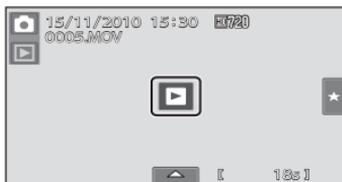
Tap the monitor during playback to display the control panel at the bottom of the monitor. The operations described below are available by tapping the icons in the panel.
