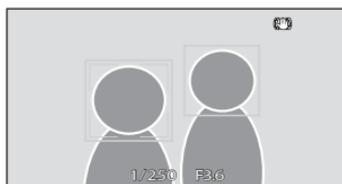
Up to three faces can be detected. When the camera detects more than one face, the double border is displayed around the face closest to the center of the frame, and single borders around the others.
