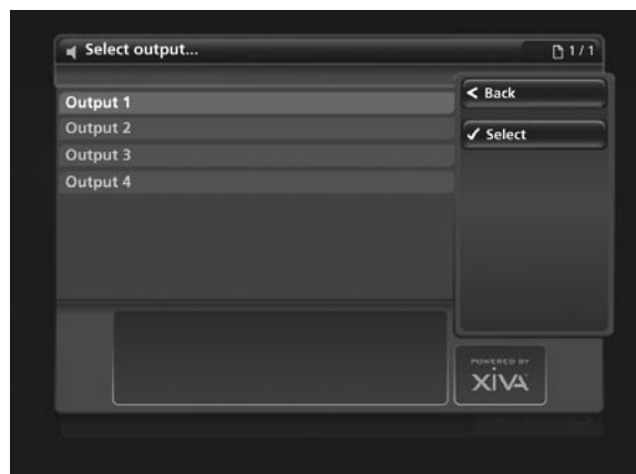
Fig. 3-20 Switching the TV user interface to control each of the DMS4's audio outputs
