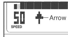
When a downward-pointing arrow appears, decrease your speed. When no arrow appears, maintain your current speed. **Important: The target speed settings are intended only to provide motivation. Make sure to pedal at a speed that is comfortable for you.**
