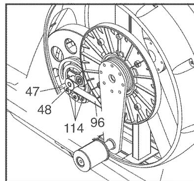
Reattach the left disc with the four screws and then reattach the left disc cover.
