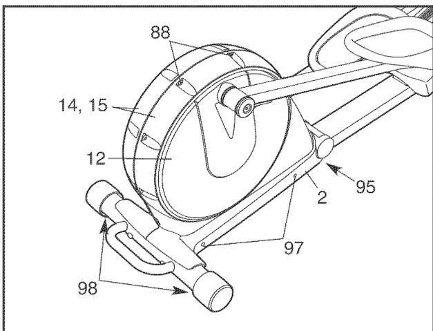
If the elliptical exerciser flexes in the center during use, turn the Center Foot (95) until the flexing is eliminated.
