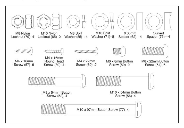
Attach the Left Front Stabilizer (15) to the left side of the Upright Frame (5) with three M8 x 22mm Button Screws (54) and three M8 Split Washers (55). Make sure that the Left Front Stabilizer is turned so the Wheel (17) is facing forward as shown.
