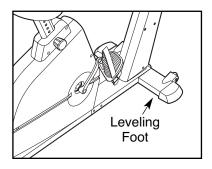
rocks slightly during use, turn one or both of the leveling feet under the front stabilizer until the rocking motion is eliminated.
