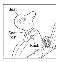
two or three turns to loosen it (if the knob is not loosened enough, it may scratch the seat post). Next, pull the knob, slide the seat post to the desired height, and then release the knob. Move the seat post up and down slightly until the pin on the knob snaps into one of the holes in the seat post. Then, turn the knob clockwise until it is tight.
