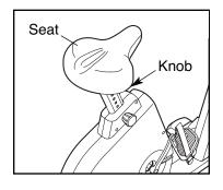
while you are sitting on it. To adjust the seat, turn the seat knob counterclockwise two or three turns to loosen it, slide the seat to the desired position, and then firmly retighten the knob.
