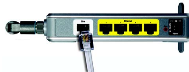
Figure 4-4: Connect the ADSL Line
