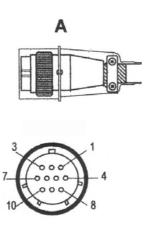
The front view of the 2 kW interconnection cable is shown above.
