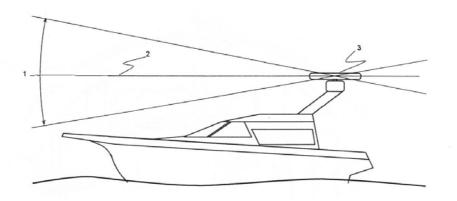
However, when the power boat is traveling at high speed, the bow rises up out of the water and if the elevation angle (trim) of the bow is raised up so that it equals, or exceeds, 50% of the vertical beam width of the radar, this can cause two problems:
