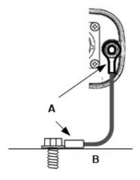
The eyelets must be crimped or soldered at both locations (A) and the method of connection to the vessel's hull is shown at (B).
