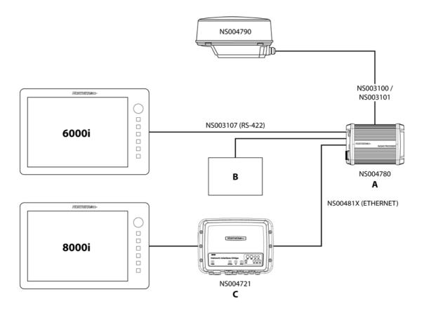
where A is the radar processor, B is the vessel's power supply (12 V DC ONLY), and C is the Network Linker (NS004721).
