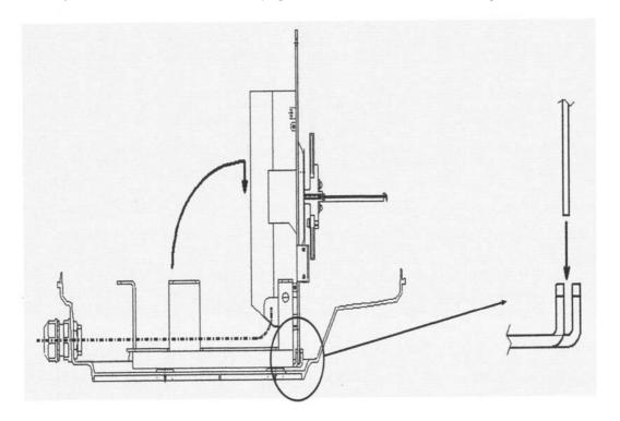
Remove the shield cover from the underside of the main unit to expose the J connector locations and ground terminal location.
