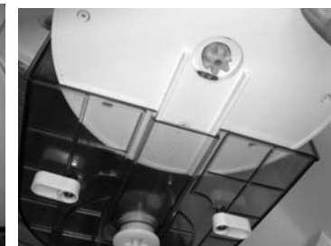
Aluminum/auger mixing mechanism in mixing chamber, and being lifted out
