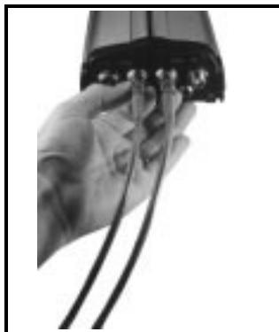
Figure 22 Removal of Connectors
