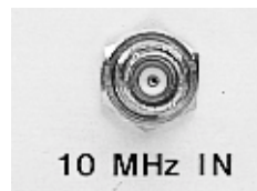
Figure 5 10 MHz In (External Frequency Reference) - Test Bed
