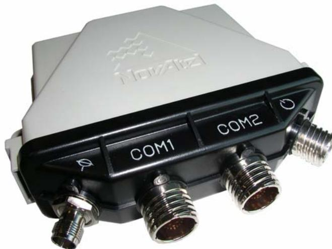
**Figure 2: FlexPak-SSII Enclosure**
