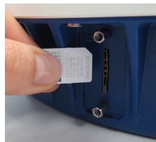
Figure 12: SIM Being Installed
