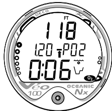
Fig. 47 - HIGH PO 2 WARNING
