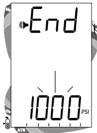
Fig. 35 - Set End Pressure Alarm
