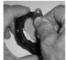
Fig. 46A - COVER REMOVAL (using tool)
