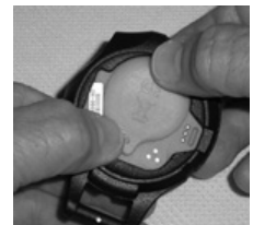
Fig. 50B - COVER INSTALL (using thumbs)
