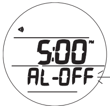
Fig. 19 - DAILY ALARM STATUS (Set, ready)
