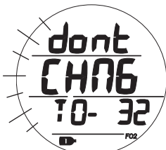
Fig. 99 - GAS SWITCH ALARM (all flash)
