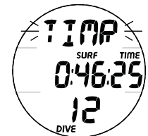
Fig. 61 - FREE SURFACE CDT ALARM
