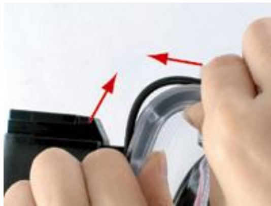
FIGURE 2: PROVIDING A LOOP IN THE GASKET
