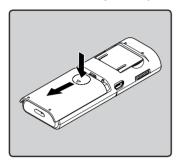
2 Insert the batteries, observing the correct ⊕ and ⊖ polarities.
