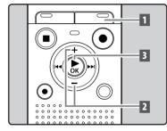
1 While the recorder is in stop mode, press and hold the CALENDAR/SCENE button.
