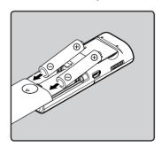
3 Close the battery cover completely by sliding to the direction (A).
