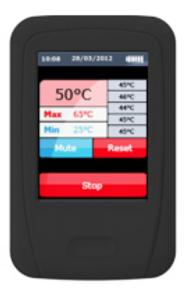
This robust easy to use handheld device takes and records temperature readings via the attached K-type probe supplied with the unit. A large touch screen, color display indicates temperature, maximum and minimum readings and will produce a graph of the data.
