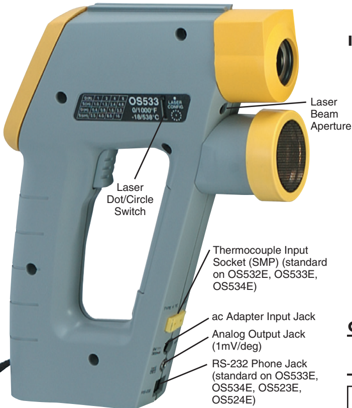
Figure 2. OS530E/OS520E Series Handheld Infrared Thermometer Various Views
