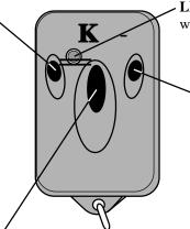
**LED Light-** Illuminates when a button is pressed.
